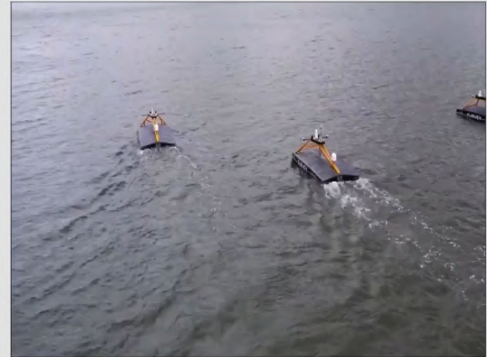
Fig. Multi-USV for bathymetric survey
